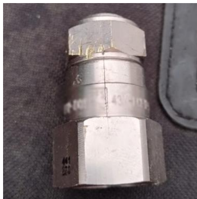
Severe hex nut marking and split body due to incorrect tool use and over torquing
